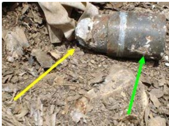
Yellow arrow points at Detonator sleeve in unarmed position Green arrow points at area where the M 77 been in contact with stone
