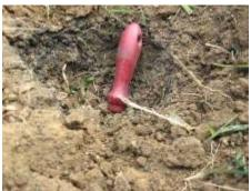
Close view of the mine blast crater no initial trench or hole can be observed
