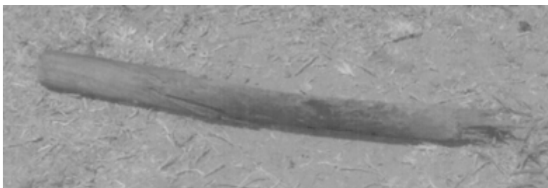
The broken handle of the pick which has been found adjacent to the accident point
