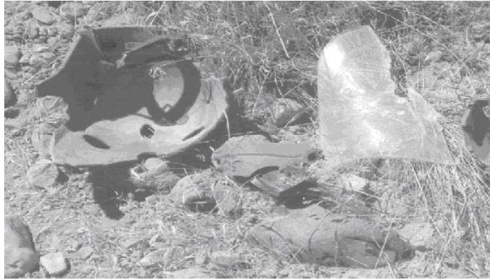
The damage to the visor and plastic helmet is shown above.
