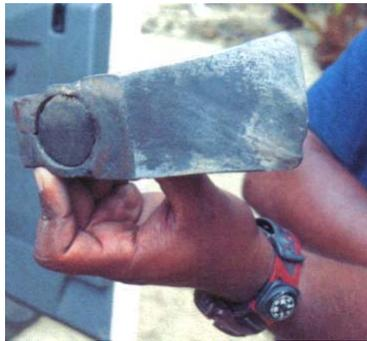
[The picture shows the head of the “Axe hammer” broken from the handle and with the corner burned off by the blast.]
