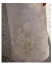
Regarding the visor (see picture) it is a timely reminder due to the email from [name excised]. The visor has absorbed and deflected the blast away from the face. You can see small fragments (Black) around the mouth area and if felt the area has been reduced by 1 to 2 mm in depth. If he had not been wearing it the blast would have hit him squarely in the face and mouth causing massive damage. I am no medic but I don't think I would have been interviewing him this morning!
