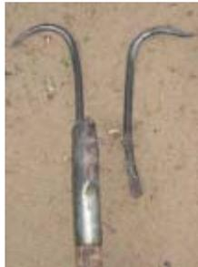
[The picture above shows the rake head with a separated tine.]
