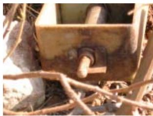
[Note that although the fuze is described as an MUV type, the pin is not the conventional winged wire sort.]
