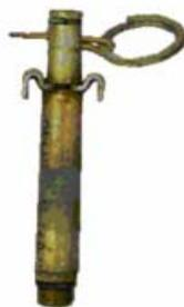
[The fuze shown was pictured in the original report and does not include the detonator – only the initiation cap. As a result it is not clear whether the complete detonator was present.]
