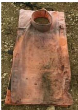
[The apron worn by the victim has a cotton cover (for comfort) and this is usually damaged in any accident. The ballistic aramid inner is not Kevlar. To raise the protection offered in “vital areas” the apron has a small, optional polycarbonate insert in the chest area. In this case the insert was in place. It is shown below along with some of the 3mm square fragments of steel recovered from inside the armour. No fragments fully penetrated the armour or the visor.]
