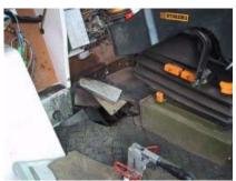
The picture above shows the floor of the cab where the steel plate covering the pedal-stem hole has lifted.
